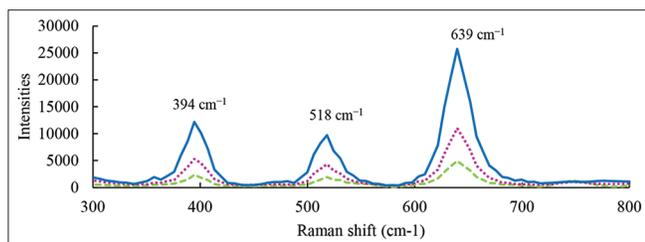
**Figure 4:** Raman spectra of film coatings at 10 min (green), 40 min (pink), and 90 min (blue) of process C
