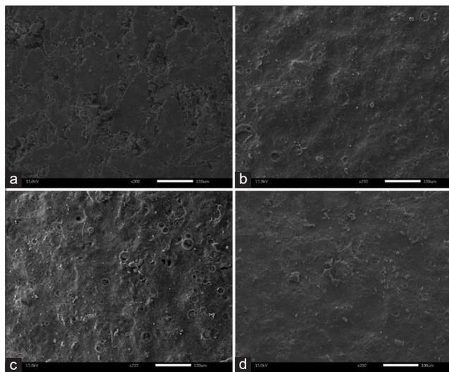
**Figure 2:** SEM images of (a) core tablet and coated tablets at the end of coating, (b) process A using pan speed of 8 rpm and spray rate of 8.2 g/min, (c) process B using pan speed of 8 rpm and spray rate of 10.5 g/min, and (d) process C using pan speed of 14 rpm and spray rate of 8.2 g/min
