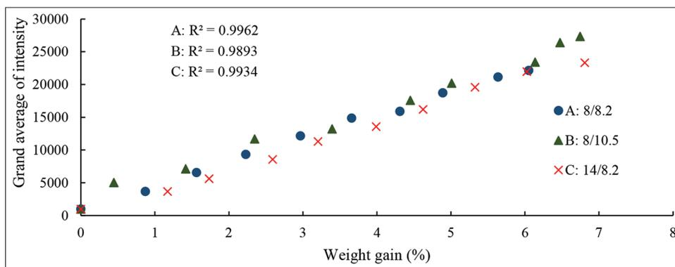
**Figure 5:** Correlation between the grand average intensity of the Raman peak at  $639\text{ cm}^{-1}$  and the weight gain
