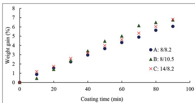
**Figure 3:** Cumulative weight gain as a function of coating time
