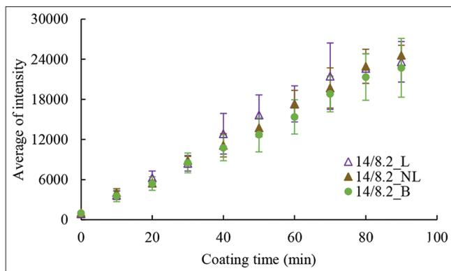
**Figure 6:** Average of the intensity ( $\pm$  SD) of Raman peak at  $639\text{ cm}^{-1}$  against the coating time of process C. L, debossed face; NL, non-debossed face; and B, band
