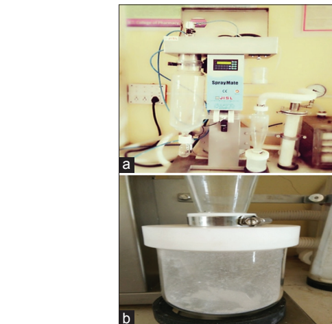
Figure 12: (a and b) Preparation of solid self-emulsifying oil formulation by spray drier
