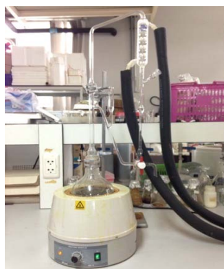
Figure 2. Clevenger apparatus for determination of volatile oil content in Piper nigrum
